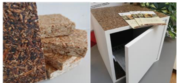
Comparison of wood-based products made of alternative adhesives or low-formaldehyde containing adhesives (left), SusBind furniture prototype (right). © Wood K plus
